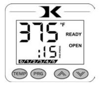
the main timer for 20. When the operator closes the press, the 5-sec time counts down. When the operator opens the press, the time setting switches to 20 seconds.
