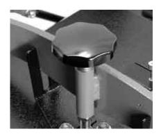
WARNING: The heat platen will become detached from the frame and drop onto the table if it is adjusted too far.
