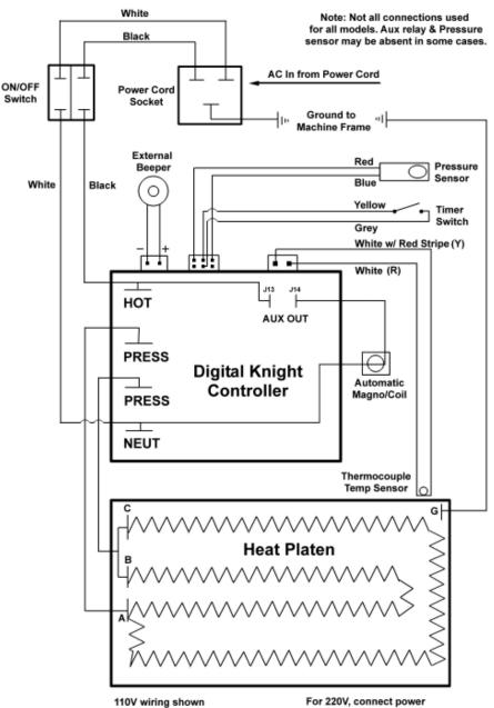
One power lead to A Other power lead to B & C joined For 220V, connect power leads to B & C, leave A empty
